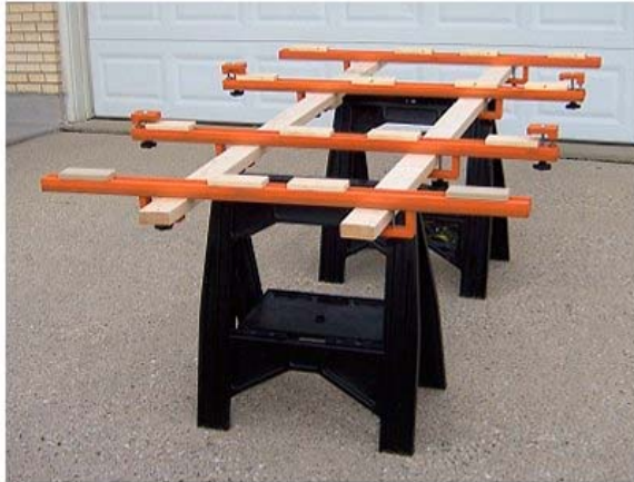
Panel Saw Setup
